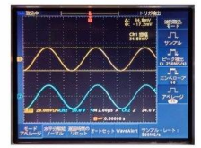
34.8mV 50Q Term (下の波形はTX直)
